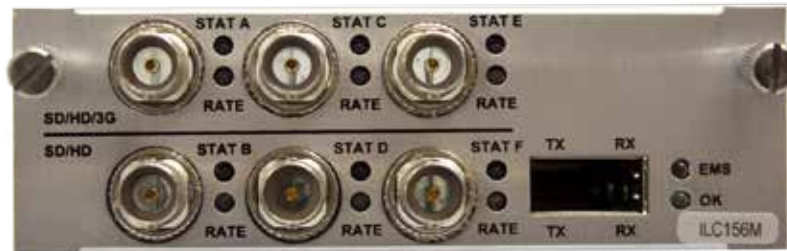
Figure 7. ILC156M BNC Connectors and XFP Socket
